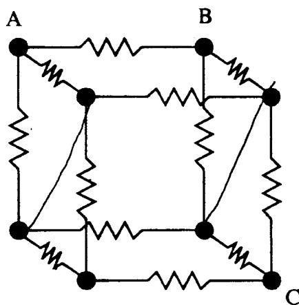
Given that all resistors are  $1\Omega$ , find the resistances between nodes:
