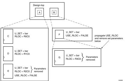
This illustration shows the use of USE\_RLOC=FALSE. The USE\_RLOC=FALSE on primitive E removes it from the U\_SET set, and USE\_RLOC=FALSE on element F propagates to primitive G and removes it from the U\_SET set.
