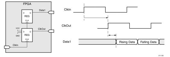
Because the regenerated clock is transmitted along with the data, the interface is primarily limited in performance by system noise and the skew between the regenerated clock and the data bits. In this interface, the time from the input clock edge to the output data becoming valid is not as important as the skew between the output data bits and in most cases can be left unconstrained.
