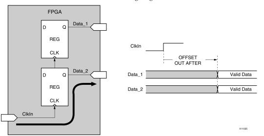
When analyzing OFFSET OUT, the timing analysis software automatically take all internal factors affecting the delay of the clock and software into account. These factors include:
