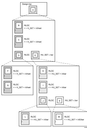
This example demonstrates how HU\_SET constraints designate elements as set members, break links between elements tagged with RLOC constraints in the hierarchy to separate them from H\_SET sets, and generate names as identifiers of these sets.
