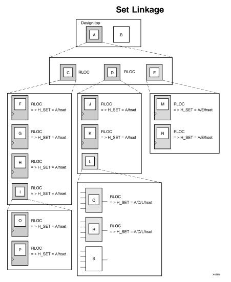
This example shows the process of linking together elements through the design hierarchy. The complete RLOC specification, **RLOC=R** *m***C***n* or **RLOC=X***m***X***n*, is required for a real design.
