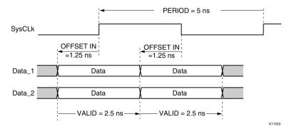
The global OFFSET IN constraint for the DDR case is defined as:
