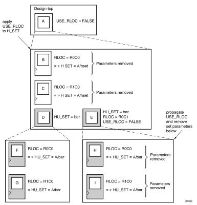
Using the USE\_RLOC Constraint to Control RLOC Application on H\_SET and HU\_SET Sets
