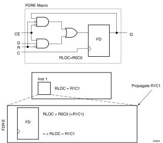
In this example, the **RLOC = R1C1** constraint is attached to the instantiation (**Inst1**) of an example macro. It is added to the **R0C0** value of the RLOC constraint on the flip-flop within the macro to obtain the new RLOC values.
