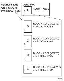
This example illustrates the process of adding RLOC values down the hierarchy. The row and column values between the parentheses show the addition function performed
