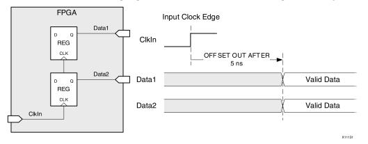
The global OFFSET OUT constraint for the system synchronous interface is defined as: OFFSET = OUT*value* VALID *value* AFTER *clock*;
