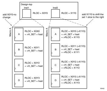
This example is a variation of the previous example. The RLOC constraint on **Inst1** and **Inst2** now link all the objects in one H\_SET set.
