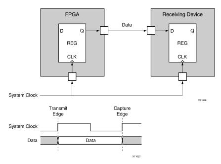
Because this interface uses a common system clock, only the data will be transmitted from the FPGA device to the receiving device.
