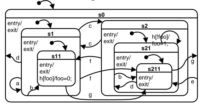
• The state machine has six states S0, S1, S11, S2, S21, and S211, and its alphabet consists of eight signals: a through h.
