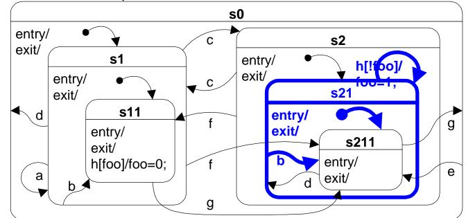
• You need to include: all transitions originating at the boundary, entry actions, exit actions, internal transitions, and the initial transition
