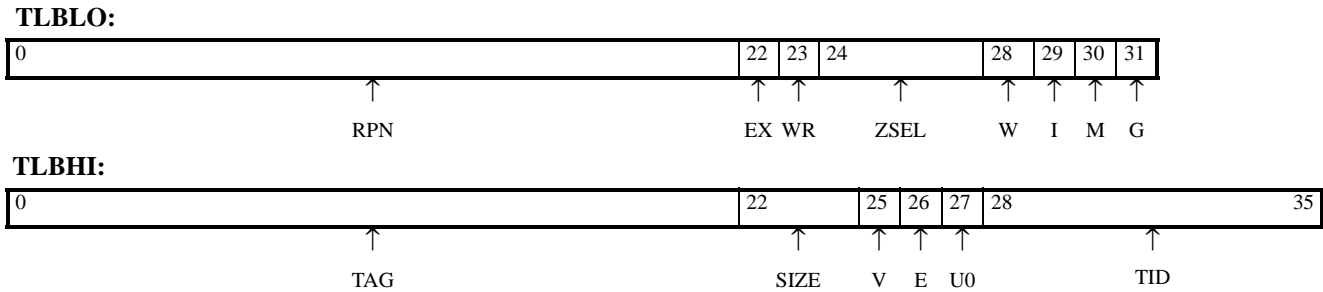
Figure 2-20: TLB Entry Format
