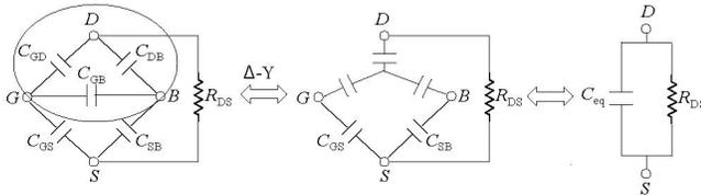
Fig 3: Equivalent RC of a MOSFET
