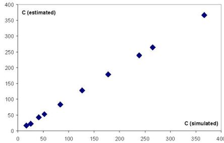
Fig 10: Fit of static decap model for ISCAS benchmarks
