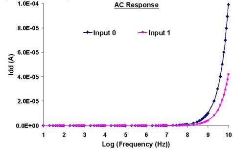
Fig 4: AC Response of a CMOS inverter
