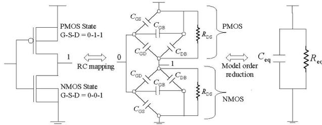
Fig 5: Analytical decap estimation for an inverter at input 0
