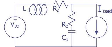
Fig 1: Canonical Power Circuit
