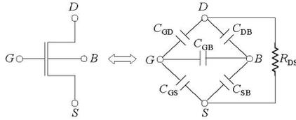
Fig 2: Resistance and Capacitances associated with a MOSFET
